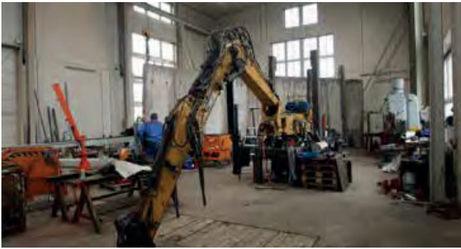
The remote controlled demolition robot, RDB 100 has been entirely developed and built in-house using the chassis of a CAT 308 D with standard components on the market.
